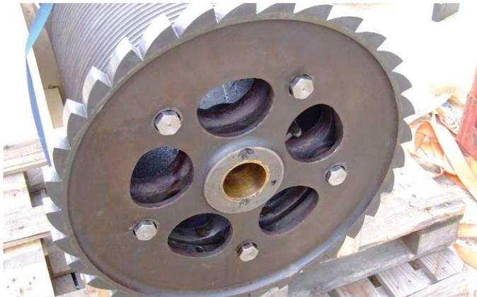
31. Ratchet wheel on hour striking barrel. At two o'clock the peg sealing an oiling hole can be seen.
