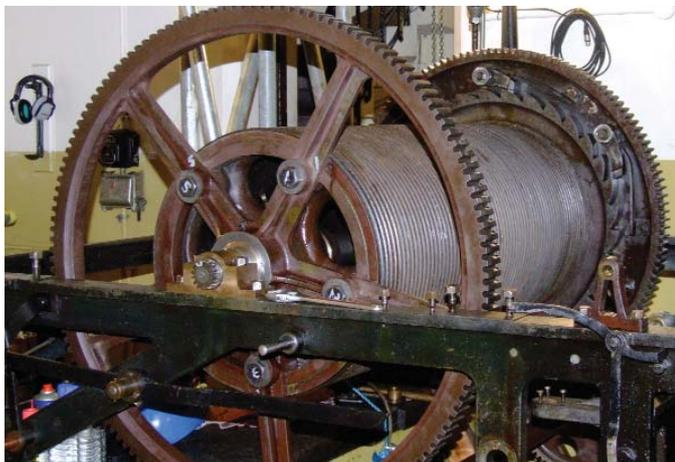
36. Fully restored, the striking barrel is back in place
