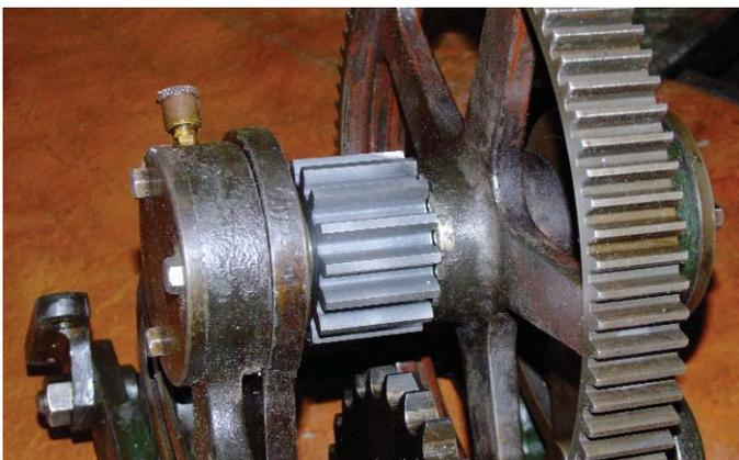
33. The new spur gear on motor-powered winding mechanism.
