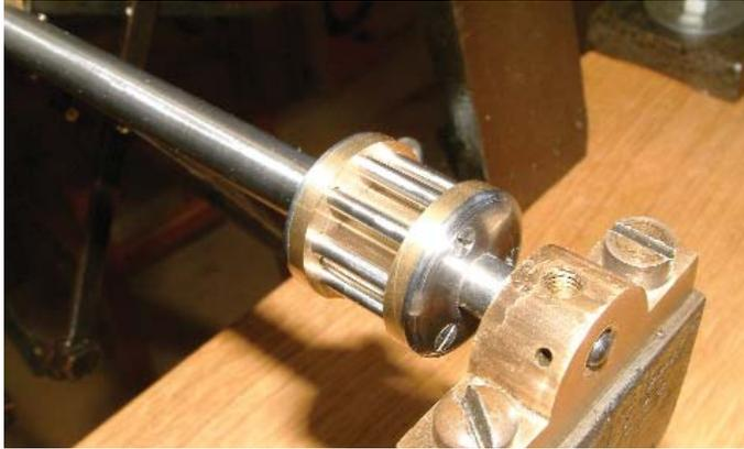
23. The finished lantern pinion and arbor made for the 'scape wheel.
