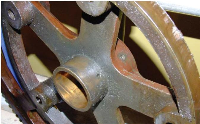
30. Bush in endplate of winding wheel. Note the oiling holes.
