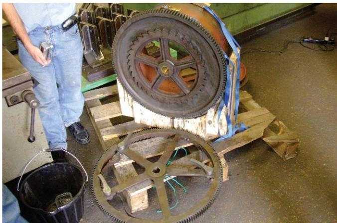
25. Going barrel and great wheel with its arbor removed. Note that three clicks are used, and the bronze bush in the barrel end.
