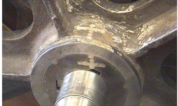
27. Repairs using cold stitches can be clearly seen looking like a row of filled holes.
