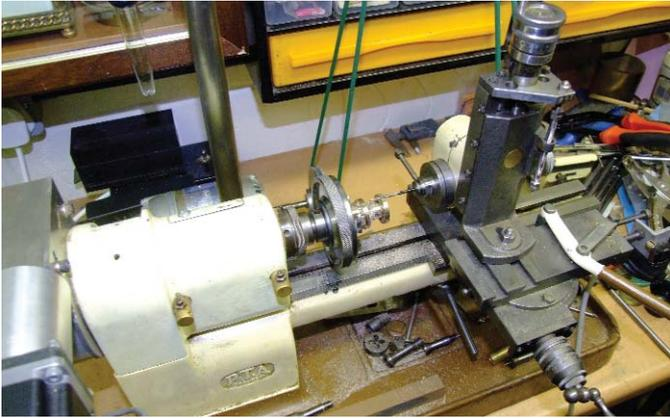
22. Drilling the lantern pinion.
