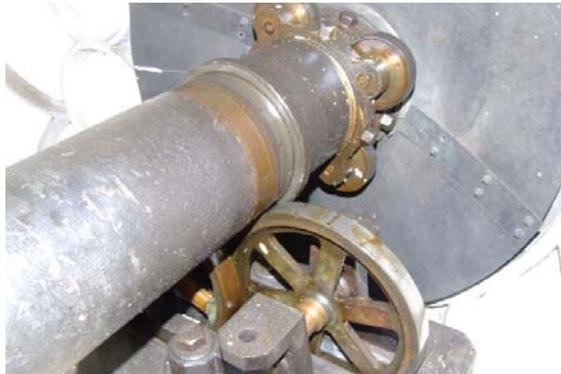
21. Friction rollers behind dial. The bottom pair of rollers take the weight of the hour tube, the cluster of four rollers mounted on the hour tube support the minute arbor.
