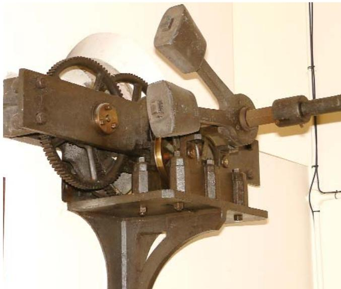
19. Motionworks inside the clock room. The Y-shaped arrangement of weights allows for precise balancing of the minute hand. Hour hand counterbalance cannot be seen here. Note one of the pair of friction wheels that take the weight of the assembly.
