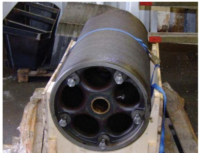
29. Barrel showing grooves to guide the line.
